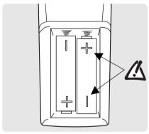
**2** Fit the batteries matching + to + and - to -.
